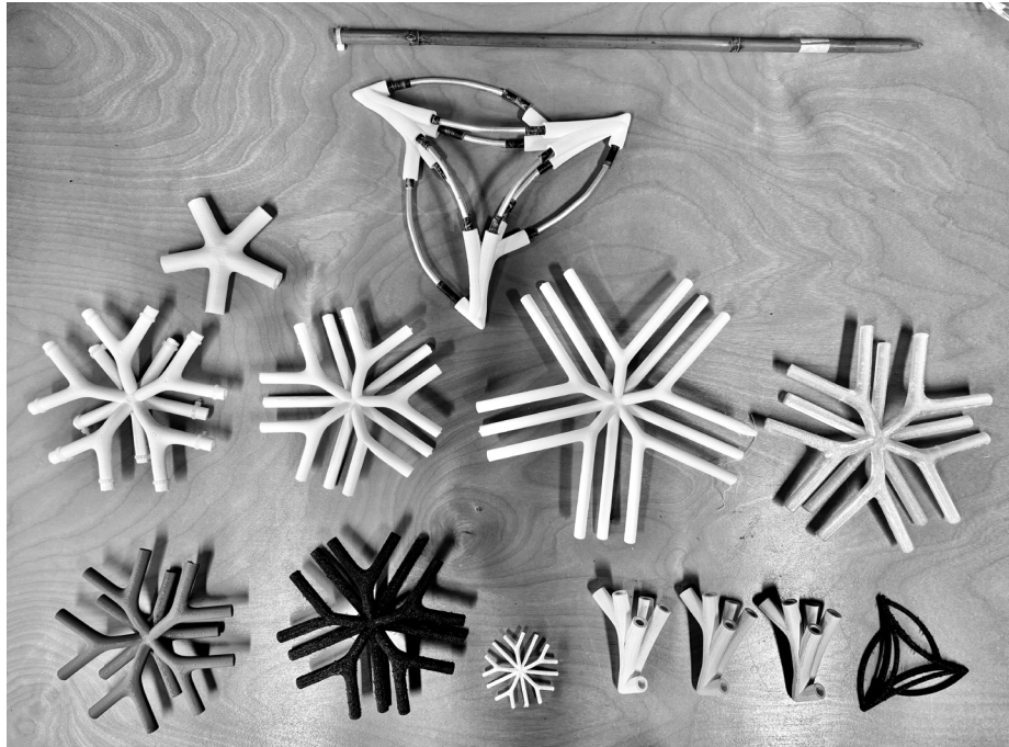
Figure 3. Rapid Prototyping Model of joinery for bamboo connections
