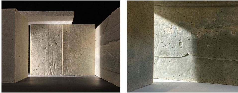
Figure 7. Scale models for a pavilion made from a geopolymer based on lime pellets
