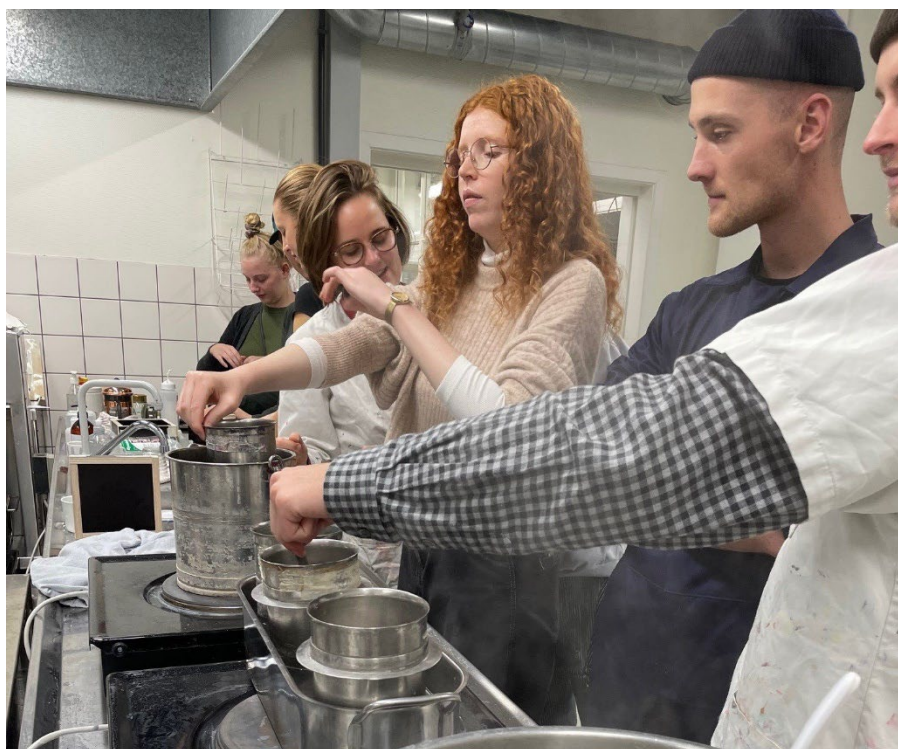
Figure 1. Students heating and agitating the starch-based mixture
