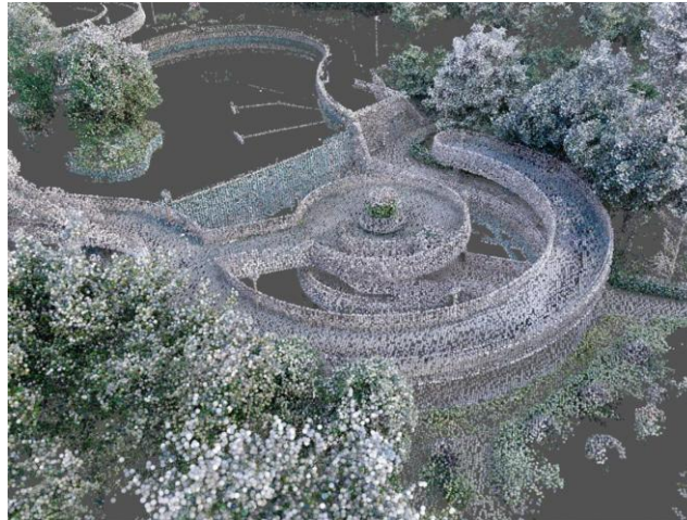
Figure 3. LiDAR scan of Shek Kip Mei Park fountain, point cloud
