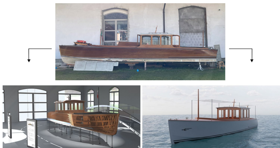
Figure 8. Picture of Ancilla before the restoration (above) and renderings showing two different projects (below). Study conducted during the course Disegno Industriale 2.2 (2022-23), Master degree in Ship and Yacht design , Department of Architecture and Design, UNIGE (credits: S. Borsi, V. Fioravanti, D. V. Jimenez, P. Marini, S. Turato, O. Giordano, V. Malagnini, S. Navisse, A. Vitali ).
