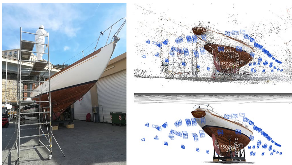
Figure 5. Digital survey through photogrammetry of Bigrin (left), the resulting point cloud and mesh (right). Study conducted during the project “Ricostruzione disegni e modelli imbarcazione Bigrin e strategie per la valorizzazione”, Department of Architecture and Design, UNIGE (2019).
