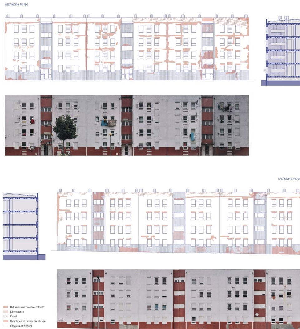
Figure 6. Identification of existing anomalies of 3 de Julho Social Housing (block 2).
