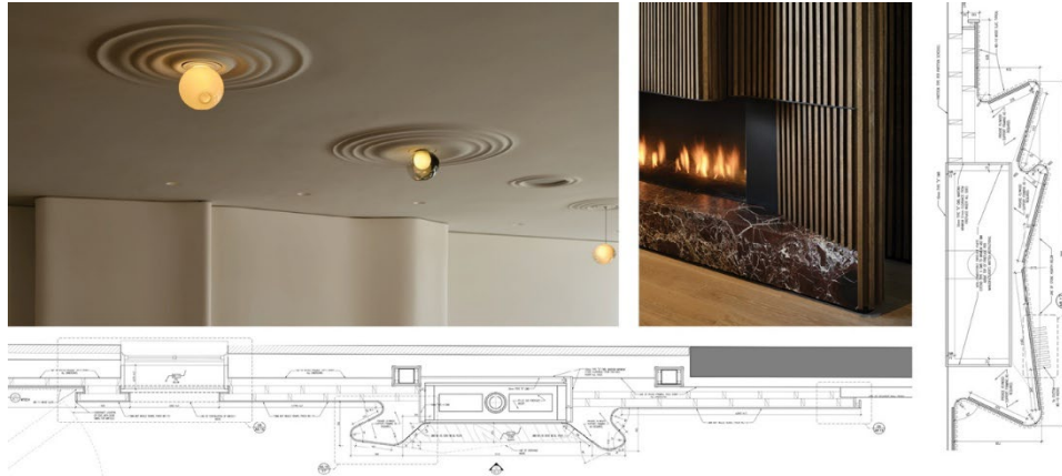
Figure 8. What was the Victorian mantle now consumes the fireplace at the exterior masonry wall whose interior lining in the form of a plaster or wood ribbed “veil” pulls away from the host masonry shell to furl and envelop the projecting hearth
