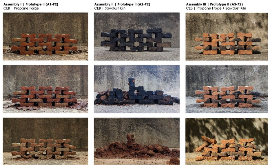
Figure 7. Documentation and observation of the decay and disintegration process of prototyped assemblies (A1-P2, A2-P2, and A3-P2)
