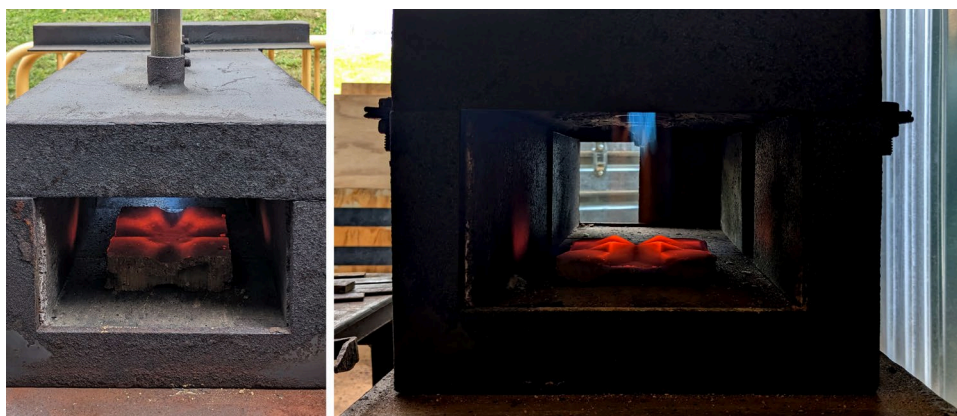
Figure 5. Block shape and geometry influencing the flow of heat and fire across the surface of prototype 2 (bp-02) and prototype 3 (bp-03)
