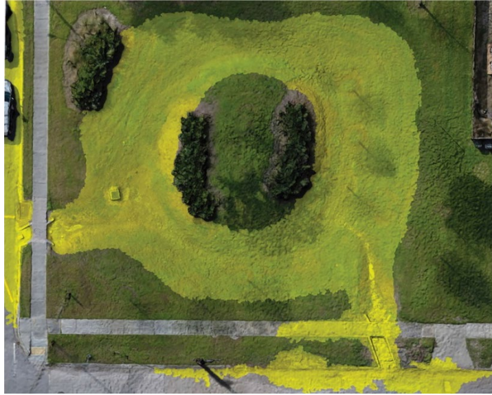
Figure 2. Digitally simulated flooded conditions at NORA rain garden case study. Image by author
