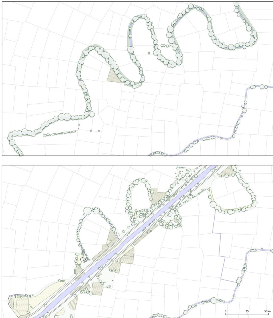
Figure 3. Channelization of a minor tributary. Years 2015 (up) and 2018 (down).
