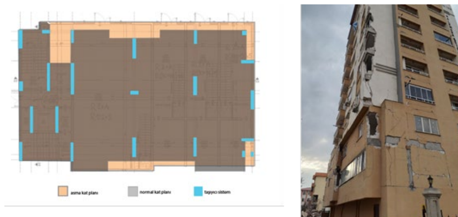
Figure 4. An example of mismatch of projection plan layouts, Kahramanmaras 2024.
