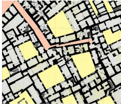
Figure 21. Floor plan of similarly scaled built form arranged around courtyards in a Tunis medina by John Habraken
