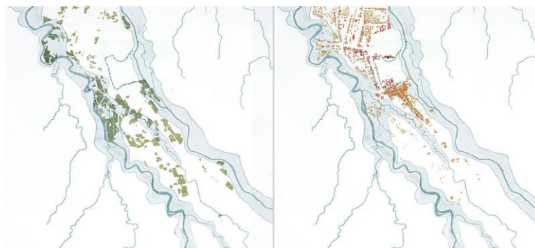
Figure 15. A reproduction of floodplain map using GLO-30 topographic data, traced with figure 8 urban tissue (green is kampung, red and orange are formal lots)
