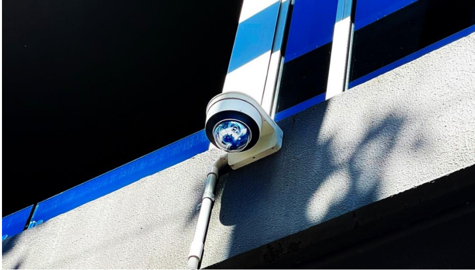
Figure 3. This PTZ (pan-tilt-zoom) surveillance camera at Grey St., South Bank, appeared to respond to my presence and observe and track my motion as I used my iPhone to record it.
