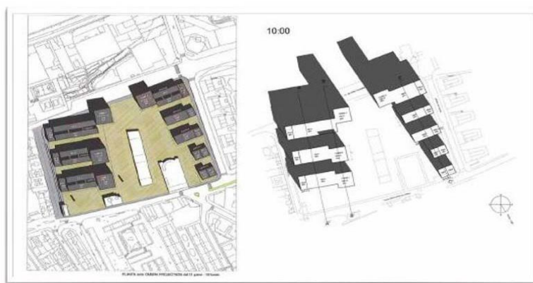
Figure 8. On the left, the calculations of the sunlight in the approved plan. On the right, the calculations by an expert. Source: Rodríguez, 2022.
