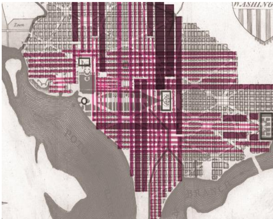
Figure 1. The District’s baroque plan, sized to accommodate monuments and buildings of state, yielded an informal network of alleys that can accommodate housing, commerce, and culture. The magenta bands indicate over-sized blocks; the background is the Ellicott Plan for the city.
