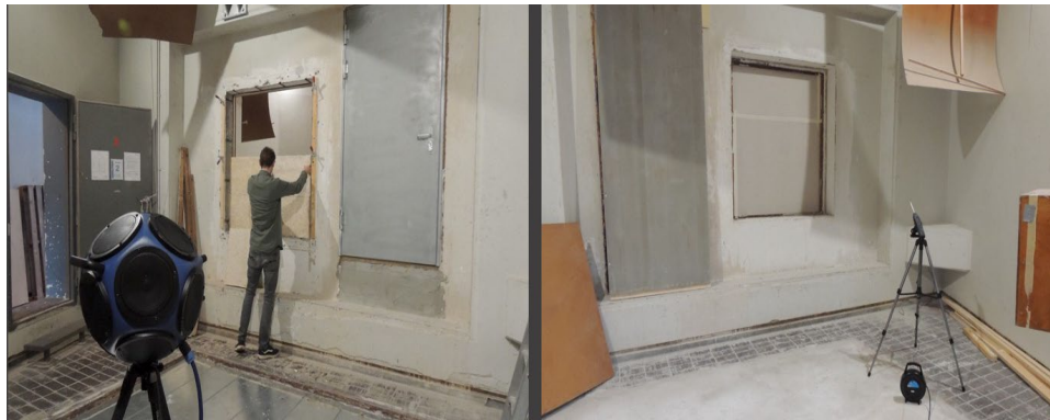
Figure 4. Set-up of sound insulation test: EN-EN-ISO 10140-2.
