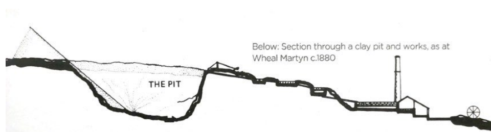
Figure 3. Wheal Martyn Trust, Section drawing showing the clay pit and works as at Wheal Martyn circa 1880
