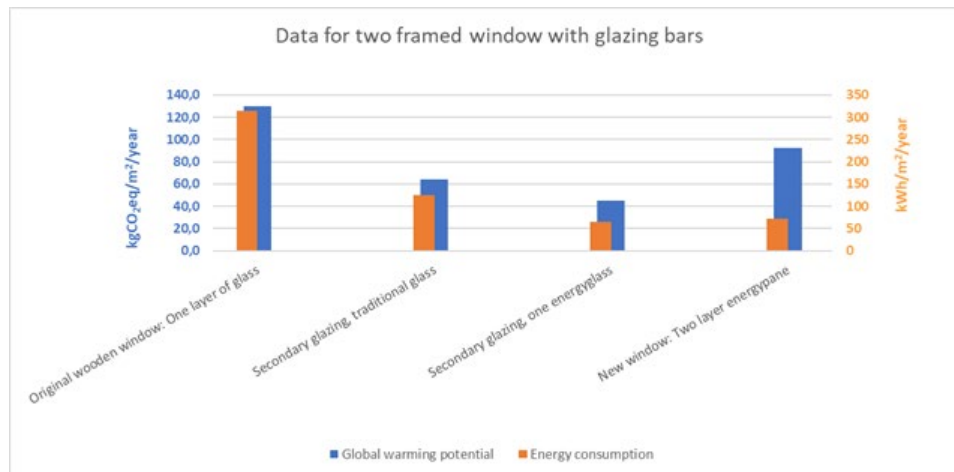
Figure 4. Comparison of Energy Consumption and LCA for a two framed traditional window. The new is made of wood/aluminium
