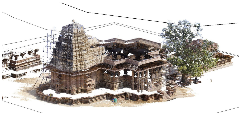
Figure 3. Point Cloud overlaid on Autodesk Revit Model
