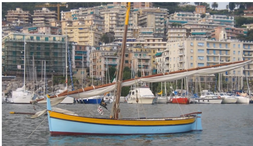
Figure 4. Alghero “spagnoletta” with lateen sail rig.
