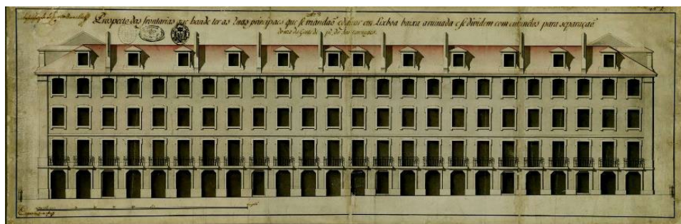
Figure 2. 1756 elevation drawing of a Pombaline block for Rua Augusta, Rua do Ouro, and Rua da Prata. 7
