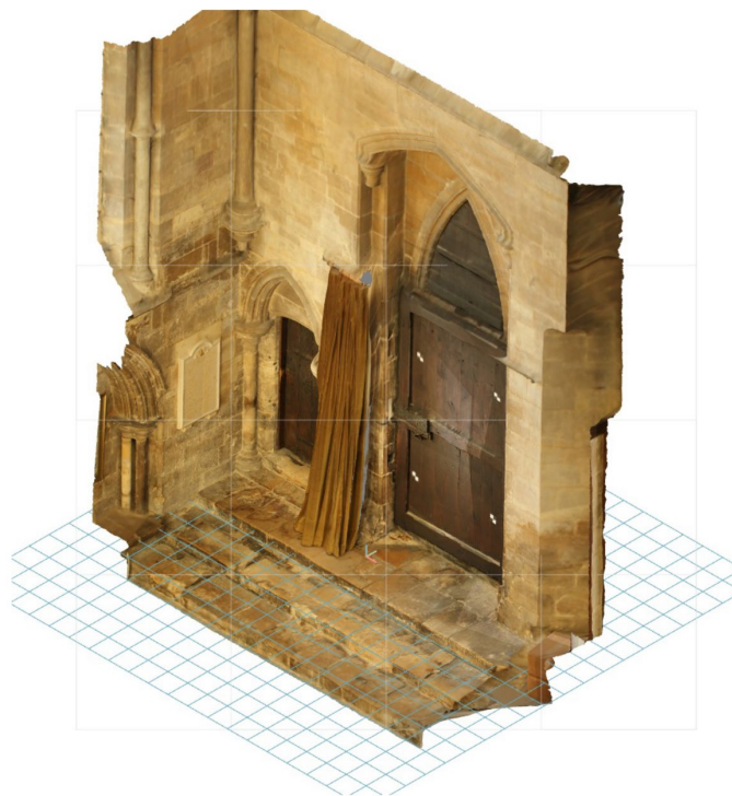
Figure 5. Photogrammetric model of the Ringers Chapel in Lincoln Cathedral, generated in Autodesk Recap Photo from photographs taken for this purpose
