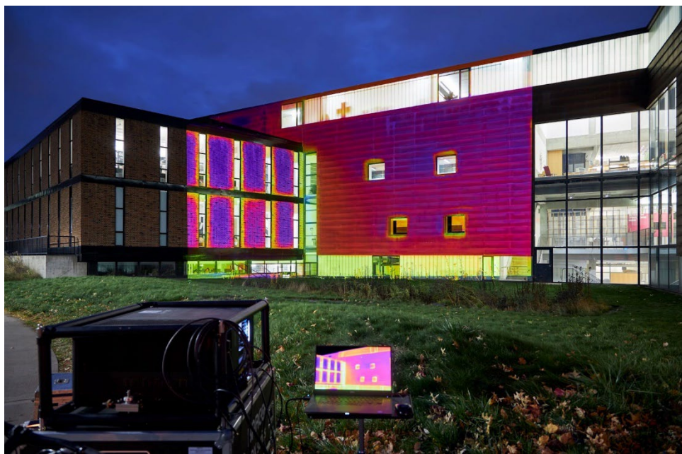
Figure 9. Projective mapping the winter thermogram on Rapson Hall (a). Photograph by Nate Anderson.
