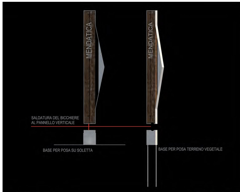
Figure 6. Technical drawing of the installation, featured with material and constructions details, applied on the single element
