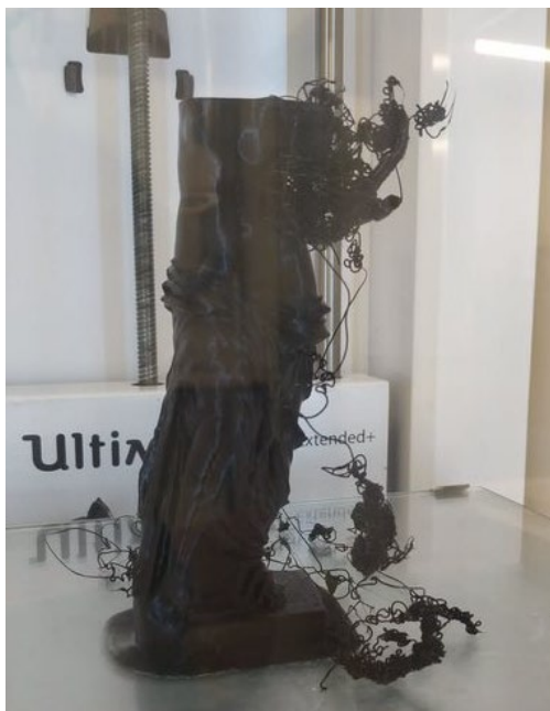
Figure 7. Failed 3D print (Self-generated Image(s), 2022)
