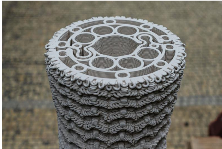
Figure 8. Continuous clay extrusion making up a monolithic interspatial structure
