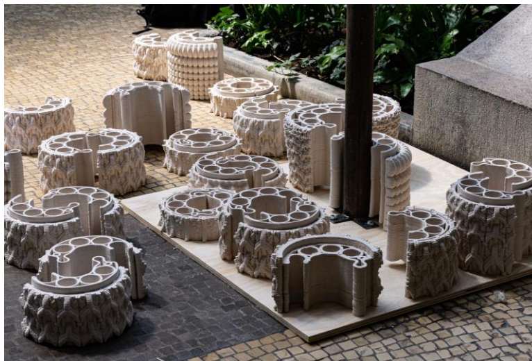
Figure 2. Column elements interlock in a horizontal and vertical plane
