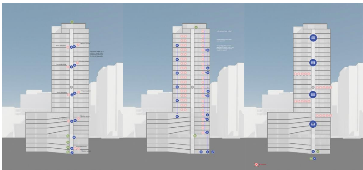
Figure 24. The FES study building populated with stickers representing components that the focus group deemed necessary or important to the wastewater hydroelectric system.
