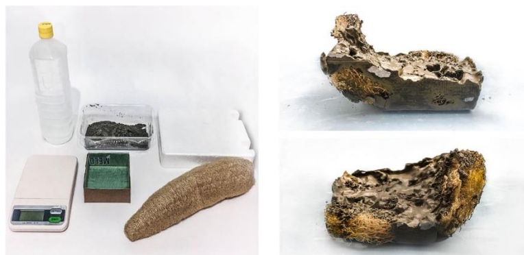
Figure 7. Documentation of loofah concrete experimentation by TSANG Ka Lai Lilian, ARCH 7182 ‘Material Diaries’, 2020
