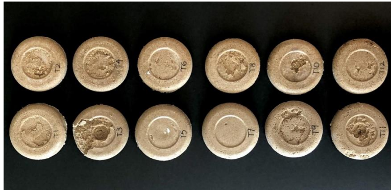
Figure 2. DIY material experiments: 'corncrete' samples by YEUNG Hei, Marco, ARCH 7182 'Material Diaries', 2020
