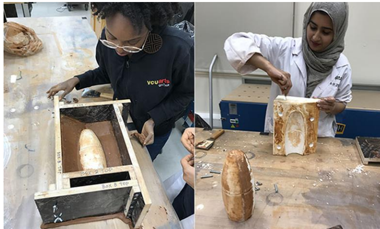
Figure 3. Slip casting with 3D-printed mold masters.
