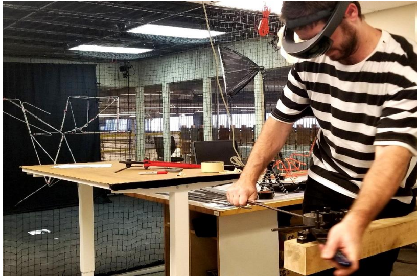
Figure 4. MR assisted fabrication utilizing holographic instruction sequences for manual fabrication of complex spatial components, enabled via Fologram.
