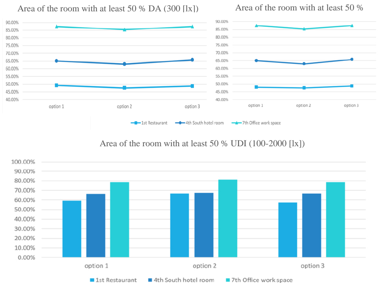
Figure 12. Comparative analysis for each floor in terms of daylight autonomy (DA), spatial daylight autonomy (sDA), and Useful daylight Illuminance (UDI))
