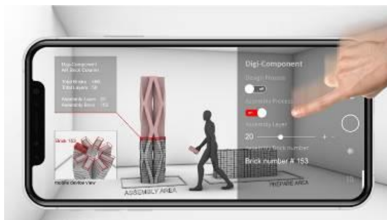
Figure 6. AR visual assembly guidance on iPhone and the mobile view during assemble.
