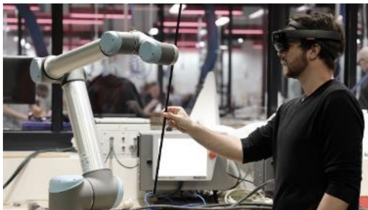
Figure 2. AR robotic operation intention in Augmented Robotics workshop (RobArch 2018). (right)
