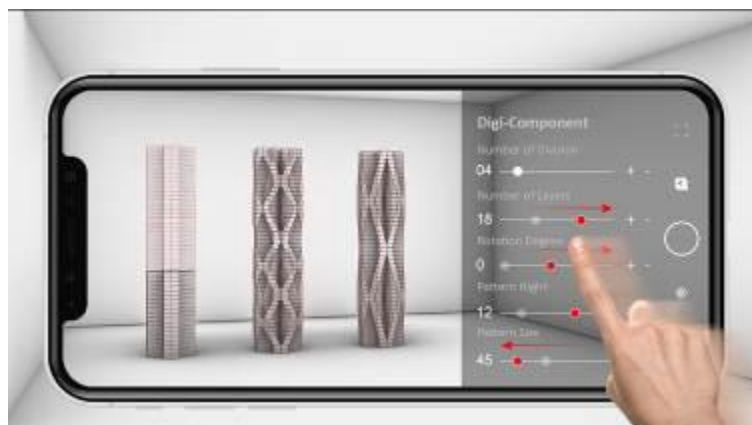
Figure 4. Interactive AR immersive design process through mobile device screen inputs.
