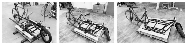
Figure 4. The initial stage for the fabrication of the PopCycle with the recycle components sourced from Geelong.
