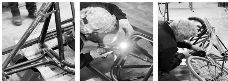
Figure 5. Assembly and welding the details of the PopCycle.
