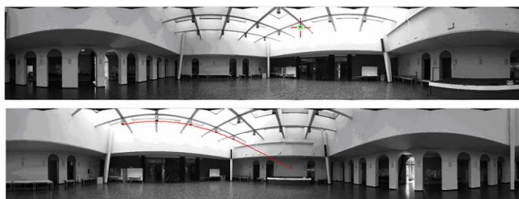
Fig. 3. Measured point in left panorama (top) and corresponding epipolar line in right image (bottom) @ Thomas Luhmann, Institute for Applied Photogrammetry and Geoinformatics, Oldenburg, Germany.
