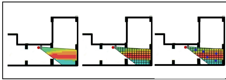
Figure 4. Proposed targeted visibility analysis of a workplace by DepthMap (Source: Authors, 2020)
