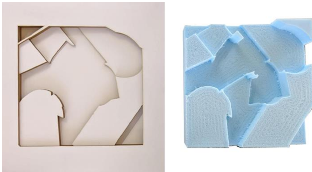
Figure 8. Exercise 5: Laser-cut and CNC mill reliefs
