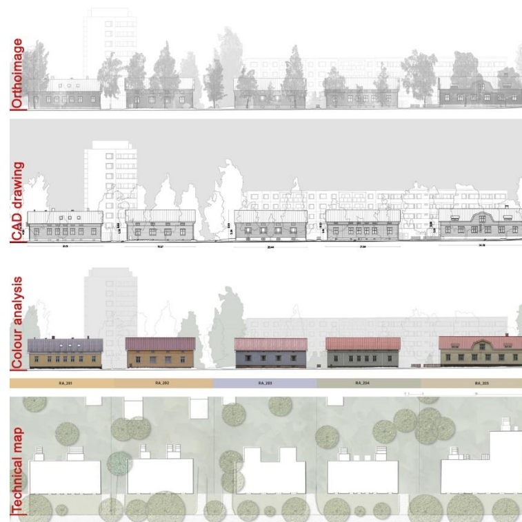
Figure 5. Extract of digital documentation elaborated for the whole neighbourhood of Raksila, technical drawings, photomaps, dimensional analysis.
