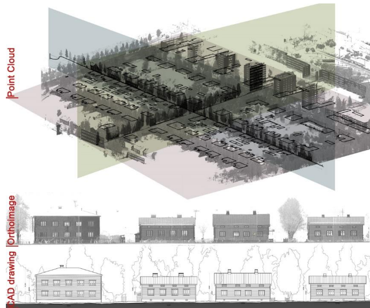
Figure 3. The process of redrawing the laser scanning survey. By exporting Ortho-images it is possible to elaborate the CAD drawings. The point cloud can be updated and used for monitoring specific situations over time.
