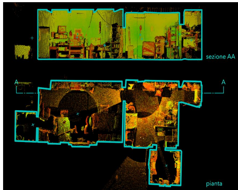
Figure 10. – Zeichen's house-shack: 2D models with point cloud overlay
