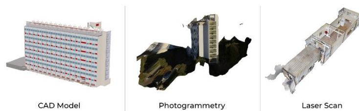
Figure 5. Types of 3D modelling techniques deployed to digitally recreate the tangible heritage of the Gordon Wilson Flats, which is embedded with intangible heritage information.
