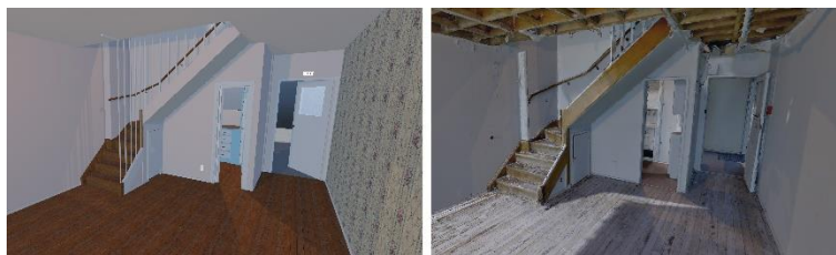
Figure 8. Left: Original colours of a flat unit (CAD model). Right: Current state of the same flat (laser-scan model textured).
